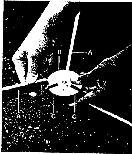
The Locked-Triangle Tripod (A) Tensioner bars (B) Lock Plate (C) Coupler slots
