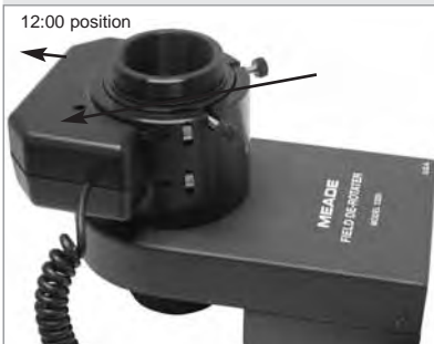
Fig. 61: Place the microfocuser over the adapter ring. Notice the orientation of the microfocuser.
