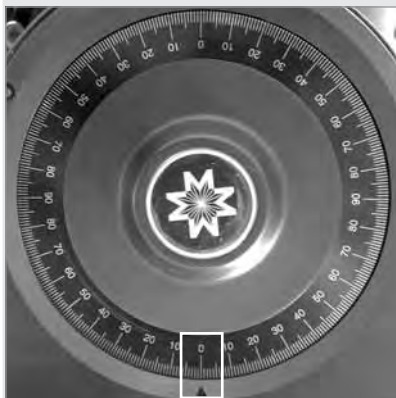
Fig. 18: Dec. Setting Circle at 0°.
