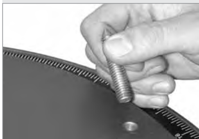
Fig. 49: Remove the pointed bolts from the drive base.
