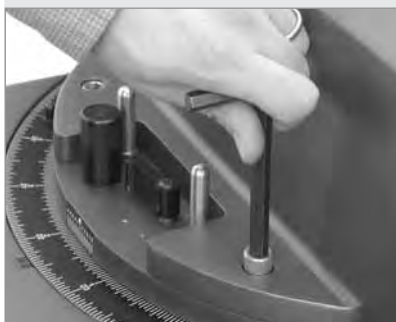
Fig. 51: Bolt the fork to the drive base.
