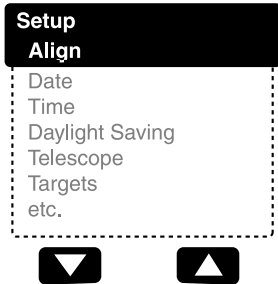
Fig. 15: Menu options display on the second line. Use the Scroll keys to move up or down through the list of options. Press ENTER to select the desired option.
