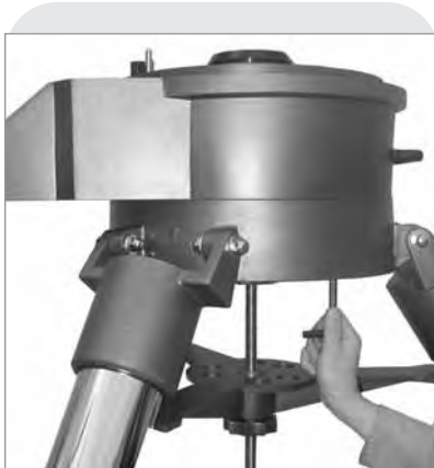
Fig. 50: Attach the drive base to the tripod.
